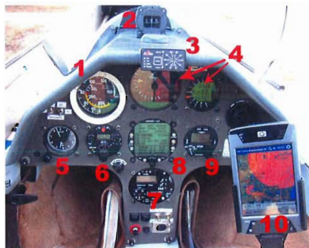
Figure 2.8. Instrument panel of a self-launch glider: airspeed indicator (1), magnetic compass (2), anti-collision alert (3), variometers (4), altimeter (5), radio (6), engine control unit (7), GPS navigation computer (8), transponder (9), moving map display (10)
