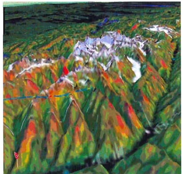
Figure 5.1. Recorded flight track on a TherMap rendered in 3D. The climbing segments (red portion of the flight track) are confirmed by the computed hot spots (brown-to-red surfaces).
